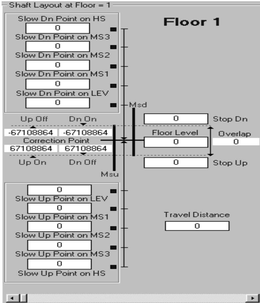
The shaft layout shows the layout for each floor level with all the corresponding settings. By using the scroll bar at the bottom, the layout for each floor can be viewed. Slow up / dn and stop up / dn points can also be changed.
