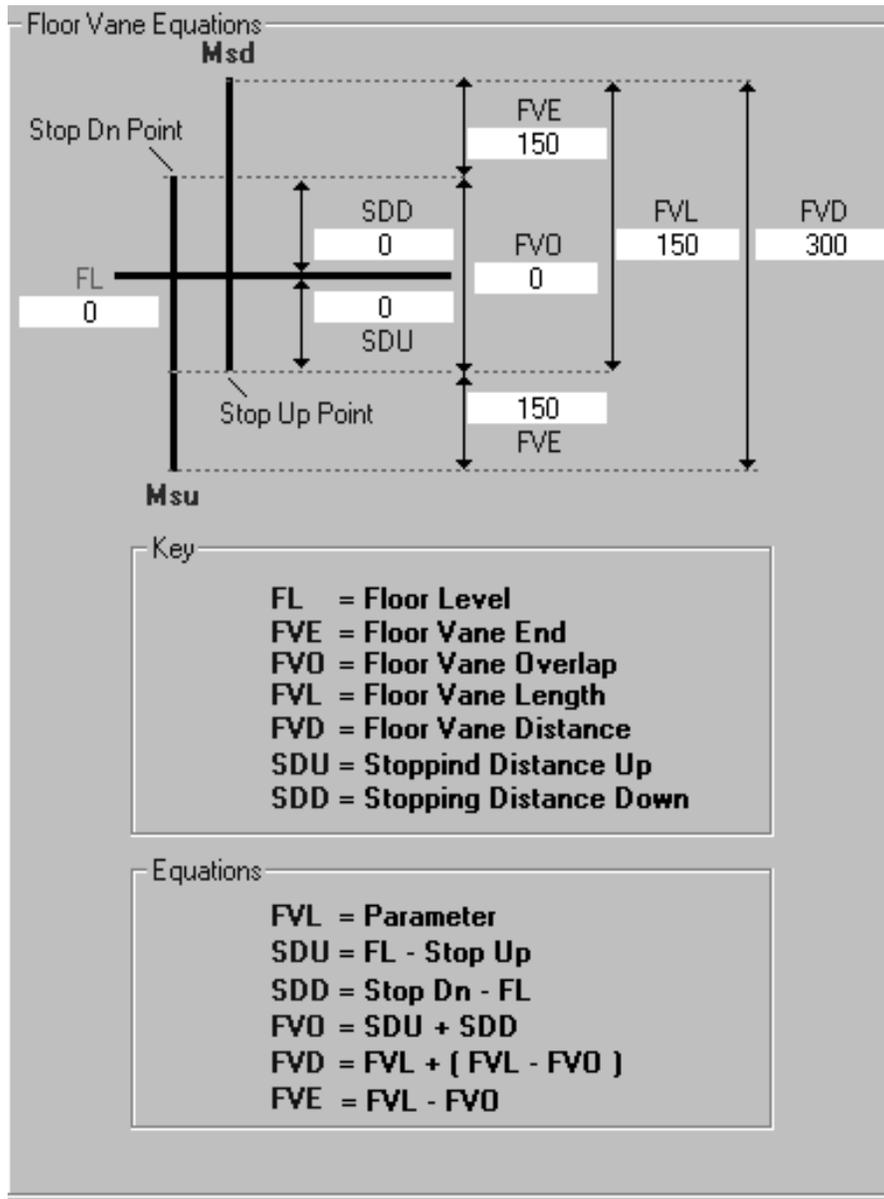
The Show Equations layout shows the equations and the results, which have been calculated by the software for that floor. The key explains the abbreviations used for the calculations.
