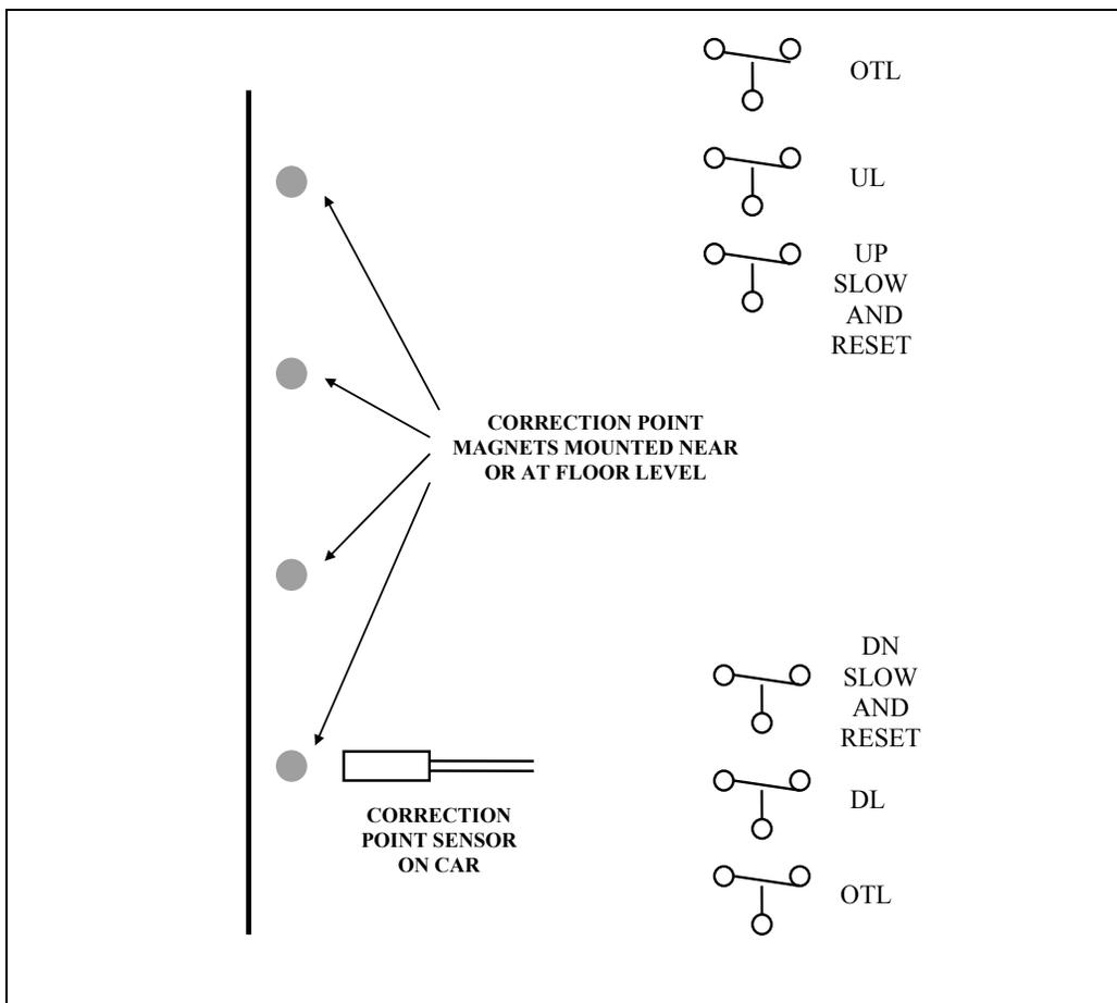
The correction point proximity switch should be mounted on the car with the distance from the magnets as shown below:
