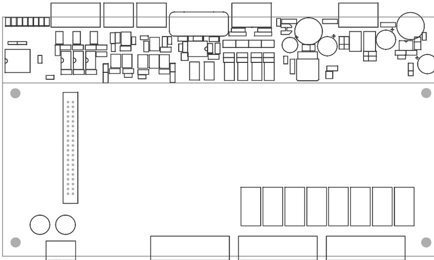
The above shows an earlier version of the shaftencoder i.e. “Positioning Device” that was external to the Skycom rack. The IOFIO16 board mounted on top of the main CPU board interfaces to the Skycom by outputs such as MSU, MSD, PX and inputs such as speed, direction, movement and resets.
