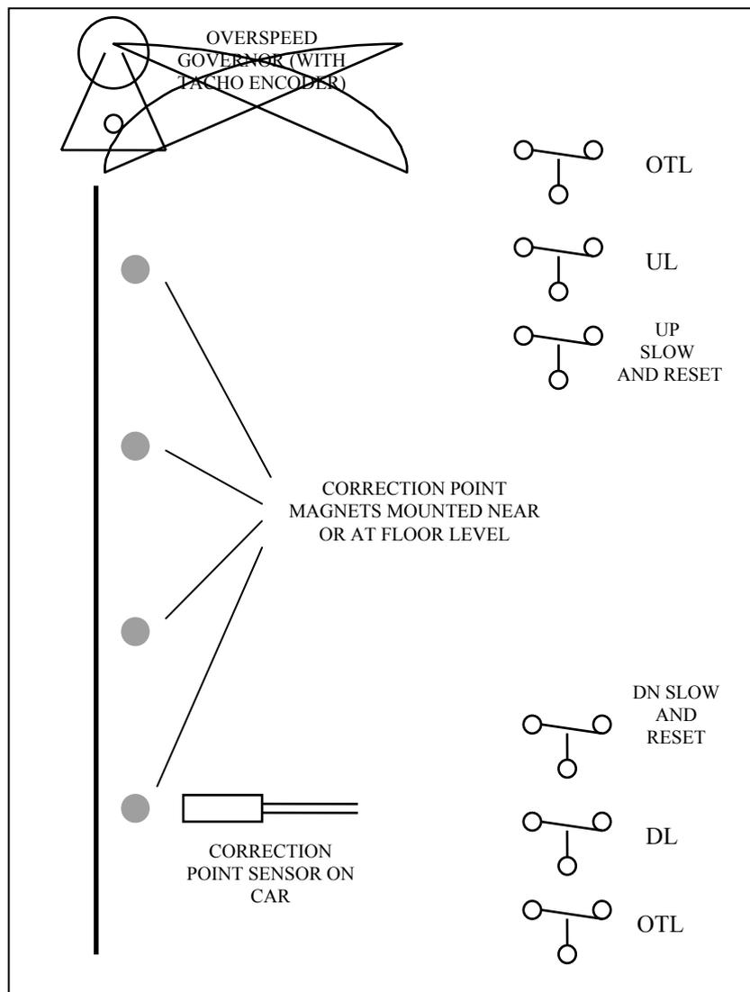
The correction point proximity switch should be mounted on the car with the distance from the magnets as shown below:-
